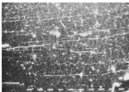
Fig. 5. Photomicrograph of tensile fracture surface of mix S, tear lines (50 \times ).
