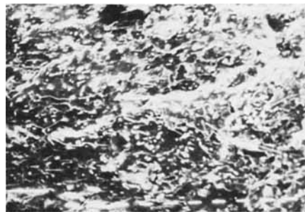
Fig. 18. Photomicrograph of tear fracture surface of mix Y (50 \times ).
