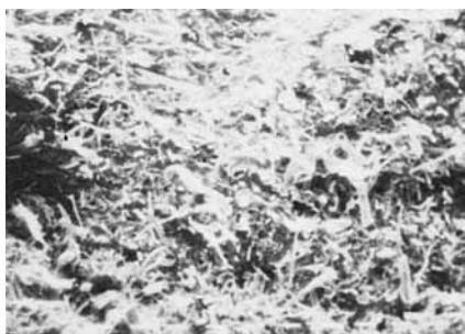
Fig. 19. Photomicrograph of tear fracture surface of mix Z (50 ×).
